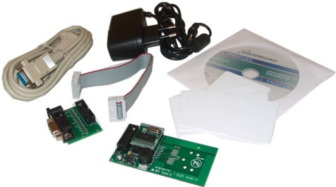
SMX1300-EK – Serial RFID Mifare Reader/Writer Evaluation Kit
